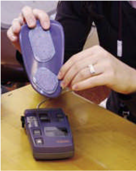
The NESS H200 can be customized for each patient, since therapists can easily reposition the electrodes, and then reprogram them using the handheld microprocessor.
